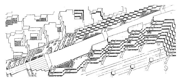
Fig. 4. Cutaway view showing coupled pan space frame and sloped street.
